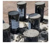
test specimens are cast, stored, and initially cured in accordance with ASTM C31, Standard Practices for Making and Curing Test Specimens in the Field.
