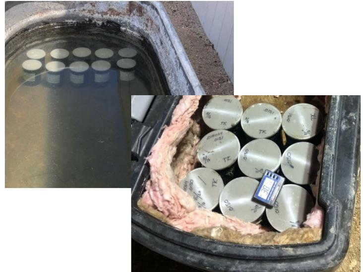
**Cylinders must be protected from direct sunlight, excessive heat, freezing temperatures and moisture loss.**
