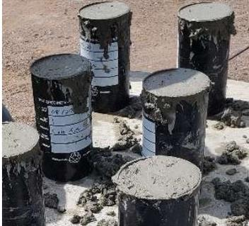
Test cylinders are used to measure the compressive strength of fresh concrete and to ensure the concrete meets job specifications. Either 6x12-inch or 4x8-inch test specimens are cast, stored, and initially cured in accordance with ASTM C31, **Standard Practices for Making and Curing Test Specimens in the Field**.
